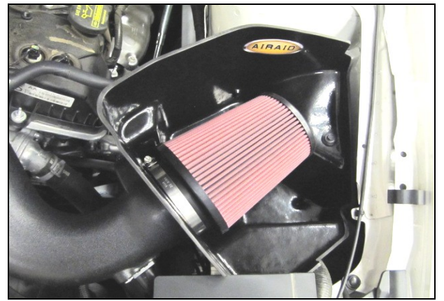
12. Install the Airaid Premium Filter (#1) onto the Intake Tube and tighten the hose clamp.
