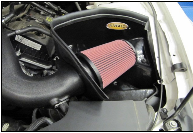
13. Install the Weather Strip (#5) onto the CAB starting at one end and working your way around.
